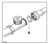
For making the connection itself, the coupling nut fitted to the machine's supply hose is designed to screw onto either a 3/4 inch gas thread spout, or to a purpose made quick-coupling tap such as the Press Block.
